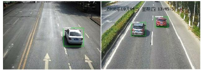
Figure 3: Examples of Vehicle Object Detection Realized by YOLOv3.
