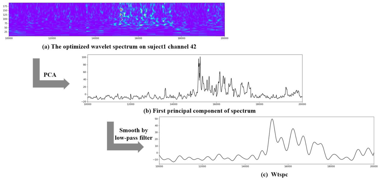
Figure 6: The Wtspc Extraction Process in Subject 1.
